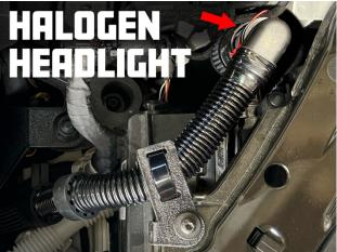
Insert the supplied wide zip tie through the two slots on the bracket. Route the SAI hose according to your headlight type and secure it to bracket like pictured. Halogen type headlight, use the supplied 8" zip tie to secure the filter to the neighboring wire loom (pointed by red arrow). Trim off excess zip tie.
