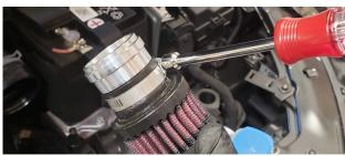
Install the supplied small filter to the billet adapter as pictured. Tighten hose clamp using 1/4" socket or screwdriver.
