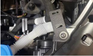
With T30 torx driver, install SAI mounting bracket using the factory screw on the headlight support bracket as pictured. The small tab goes on the left side of the triangle mounting surface. Press the tab against the headlight support bracket while tightening the screw. Snug tight.
