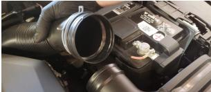
Loosen spring clamp and unplug hose from intake box. Use channel lock or spring clamp pliers.
