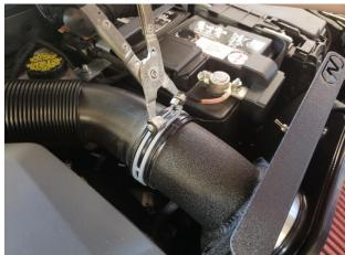
Connect factory hose until it 'pops' over the pipe and reinstall spring clamp.
