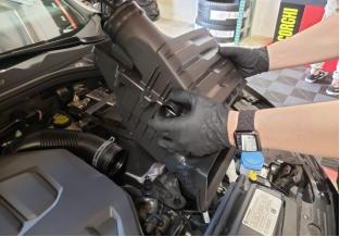
Remove airbox assembly by pulling it straight up. There are three rubber grommets that need to pop off, may require a little effort.
