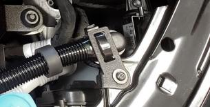
Insert the supplied wide zip tie through the two slots on the bracket like pictured. Swing over the SAI hose so the filter sits behind the headlight and points downward. Tie the SAI filter assembly to the bracket and cutoff excess zip tie.
