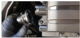
Remove secondary air injection (SAI) hose by squeezing the clip at 3 and 9 o'clock and pulling at the same time.
