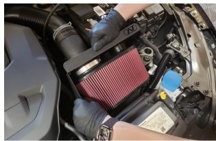
Install NEUSPEED P-Flo assembly. Make sure the (3) bottom grommets are seated completely over the posts on battery tray.
