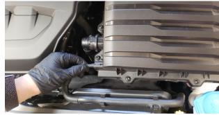
Remove vacuum hose completely on both ends. Pay attention to the end on manifold side, you will be reconnecting the supplied vacuum hose to the same fitting.
