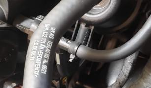
11. Connect vacuum hose to intake manifold and secure hose with supplied zip tie.
