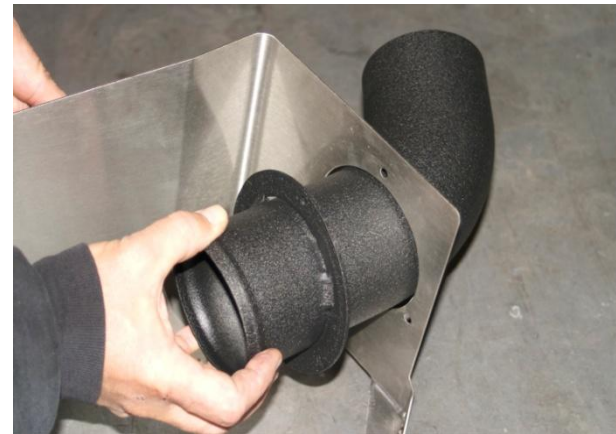
17. Remove rubber grommet from lower air box and install into hole of P-Flo bracket as shown.
