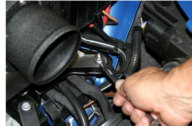
17. Remove rubber grommet from lower air box and install into hole of P-Flo bracket as shown.
