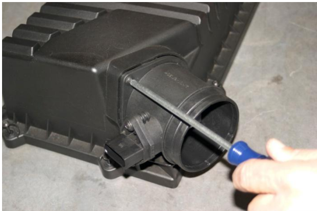
7. Unscrew and pull-out MAF from air box lid.
