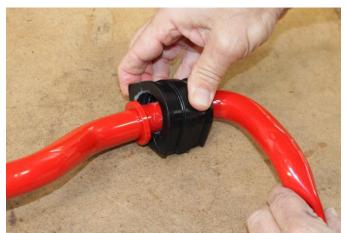
7. Apply supplied bushing grease to the inside of urethane bushings and install on the outside of stop washer on *NEUSPEED* Anti-Roll Bar.
