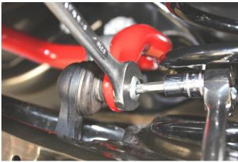
9. Attach end-links to *NEUSPEED* Anti-Roll Bar using original nuts. Torque to 48Nm (35 ft-lbs). **NOTE:** Forward hole attach end-link with suspension at full droop. Rearward hole attach end-link with suspension loaded.
