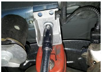
4. Support rear exhaust muffler and using 13mm socket remove the rear hanger bolts from sub-frame, one on each side.
