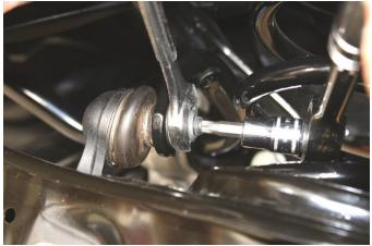
2. Disconnect end-links from original anti-roll bar by securing ball joint stud with M6 Triple Square or 5mm hex key wrench and loosening nut with 16mm wrench.
