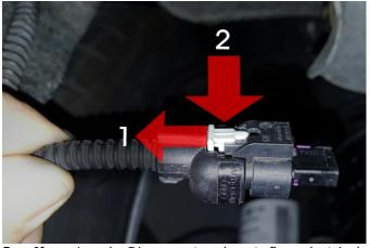
5. If equipped; Disconnect exhaust flap electrical connection on both motors and wire support clips from hanger mounts. To disconnect connector: (1) Pull out locking Grey tab. (2) Squeeze Grey tap to unlock then pull to disconnect.
