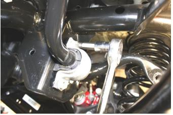
3. Remove the four bushing clamp mounting bolts using a M10 Triple Square or 8mm hex key wrench and remove original anti-roll bar from vehicle, then remove the factory bushing clamps to be re-installed.
