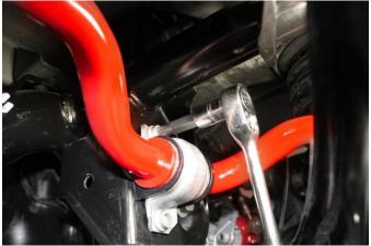
8. Install *NEUSPEED* Anti-Roll Bar using original clamps and bolts to sub-frame. Torque bolts to 20Nm (15 ft-lbs + ¼ turn).
