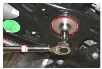
5. Torque bolt to 100Nm (74 ft/lbs) + 1/4 turn.
