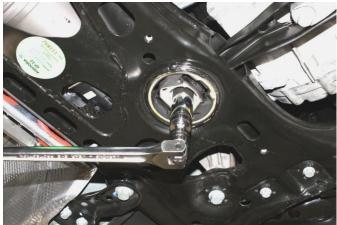
2. Unbolt and remove the 21mm hex bolt from torque mount in sub-frame.
