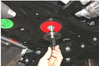
4. Install factory bolt through SS Cup Washer and tighten into mount.
