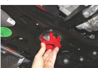
3. Use Silicone spray on urethane insert to ease installation, match up to rubber mount and push up until fully seated.
