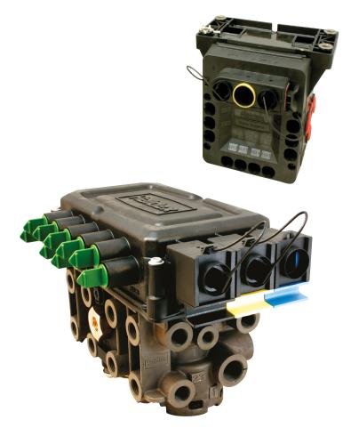
Independent EBS for full, semi and centre axle trailers. The full EB+ Gen3 3M system consisting of a Gen3 2M Master and a 1M Slave (3 modulators in total), 4 sensors, more auxiliary connections than standard, integrated stability, maximum flexibility.
