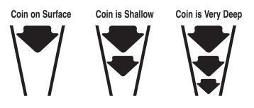
Objects other than coins will still register on the 3-segment depth scale, but the depth indication will be relative. For example, all 3 segments illuminated could indicate a coin buried 9" deep, but could also be a very large object several feet deep. Use the Depth Indicator in conjunction with the Conductivity Arc to gain more information.
