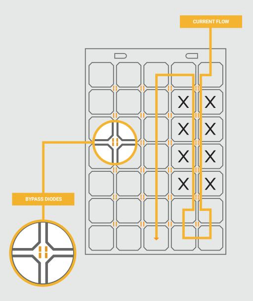
Consider getting solar panels that have bypass diodes. Some panels don't come with any, and most come with just a couple on a panel-but what would be best are bypass diodes on every cell.
