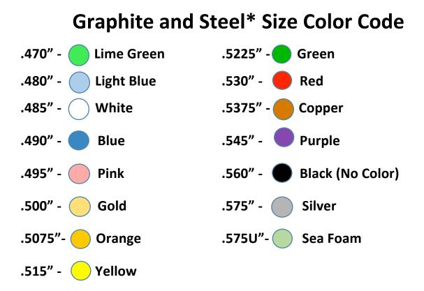
\*Steel Applications - .575" & .575U = .600" Steel, .560 = .580" Steel, .545 = .560 Steel
