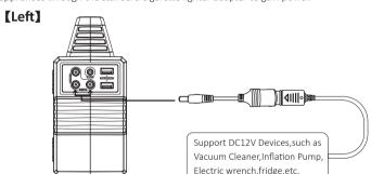
X Note: Because the battery is chemical product, voltage drops with capacity, the DC output voltage of this product is in the range of 9~12.6V, the maximum output current is 15A. If the DC12V appliance you connect does not have the voltage stabilizing function, when the DC voltage drops with the decline of battery voltage, it may cause the informal of appliance, please stop use it.
