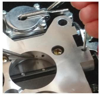
Some high performance carburetors come with an exterior **Secondary Idle Speed Screw** that you can adjust from the top with the carb installed, just like the Primary Idle Speed Screw. This will make equalizing the throttle opening amount between primary and secondary much easier, which should be done in high performance applications with 4 Corner Idle carburetors.
