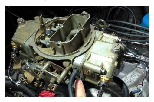
Some carburetors will have 4 Idle Mixture Screws, 2 in the primary metering block and 2 in the secondary metering block like this (which is called a 4-corner idle).
