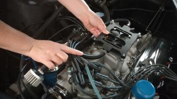
8. Place another large 4-hole gasket in top of the POWERBLAST SPACER and use Zip Ties to secure the inlet hoses to heater core hose (or other line or bracket) to ensure the inlet hoses do not bend so much that they collapse at any point.
