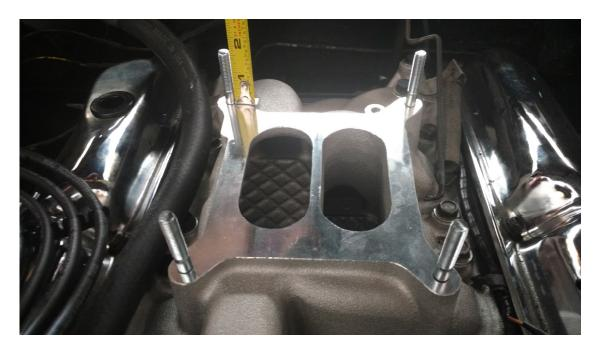
2. Install a new base gasket onto the intake manifold. Make sure all meeting surfaces are clean, flat and dry. Cover the intake manifold openings until the next steps are complete and you are ready to install the SPACER. (On a single plane manifold, an open bottom gasket can be used)
