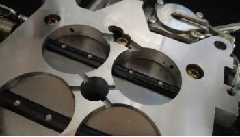
If you are running a **high performance or "Rumpy" camshaft**, which requires a higher engine idle speed (around 900-1000 rpm), your carburetor could possibly have larger than normal transfer slot exposures on the primary venturis, with the throttle blades at the previously required idle position - as shown in the photo below left.
