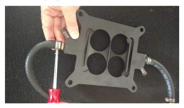
5. Check to ensure that the POWERBLAST SPACER fits flat to the bottom of the carb with a 4-hole gasket in between them, and with no interference caused by the hose and clamp connections. If you are running a hose to the rear of the carburetor's base plate, you will need to rotate the clamp for that hose so that it does not interfere with the POWERBLAST SPACER's extension, hose and clamp per this photo.
