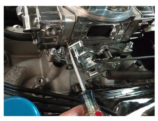
18. Your engines idle RPM is probably now much higher that when you started tuning, so you should adjust the Idle Speed Screws again as needed to set the idle speed to a normal range for your engine.
