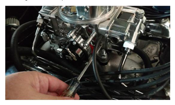
20. If when turning any one of the remaining Idle Mixtures Screws in, the RPM goes up and then back down again, back-off this screw until the RPM goes back to the point when it was highest. Then, go back to the earlier Idle Mixture Screws and turn them back out slightly to match this new setting, so that they are all the same.
