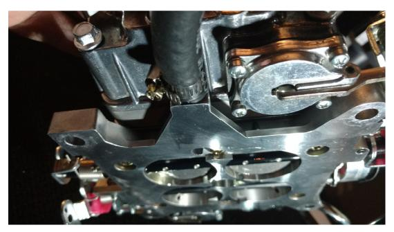
7. Install the complete POWERBLAST SPACER assembly onto the intake manifold with new base gasket and with the air channels of the SPACER facing up.
