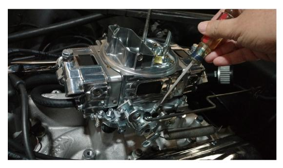
19. Now set all of the Idle Mixture Screws to the same point – one by one, as this first Idle Mixture Screw's new setting arrived at in step17.
