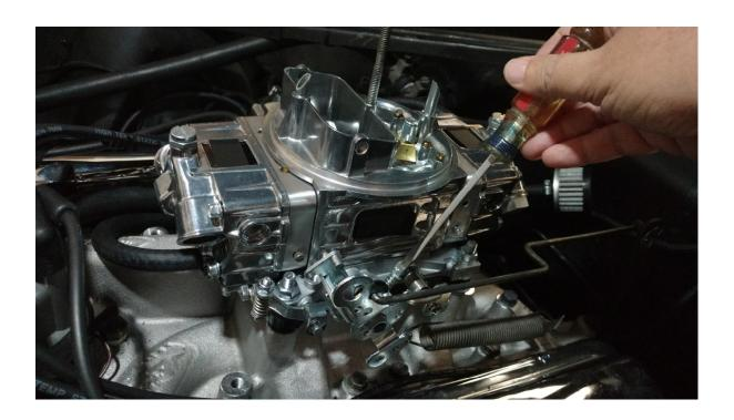
Some carburetors will have 2 Idle Mixture Screws – one on each side of the primary metering block (which is called a 2-corner idle).
