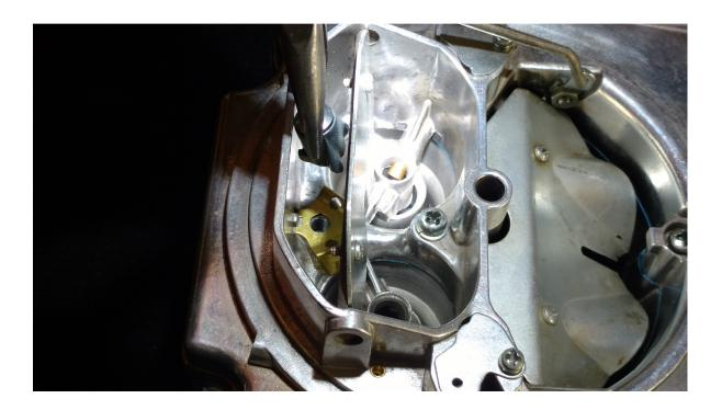
6. While holding the *POWERBLAST PLATE* centered and firmly in place, only slightly tighten the retention screw and check the alignment of the Accelerator nozzle and the *POWERBLAST PLATE*. The nozzle and *PLATE* should be aligned so the nozzle discharge holes line up with the exit holes in the plate, and the *POWERBLAST PLATE* should be positioned for equal spray into each venturi.
