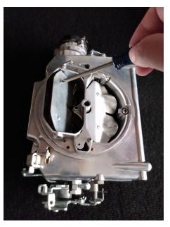
2. Fully loosen the accelerator pump nozzles retention screw.
