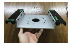
The RGS Router Base Plate is now assembled. Next are the Gantry Rails that create the "Bridge Assembly" of the system.
