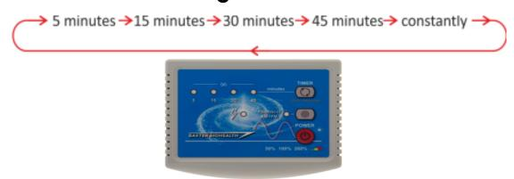
Choosing a time is required by a short press on the timer button. Shown above, the timer is switched in a circle. The chosen time is indicated by the lighting of the corresponding LED on the front panel of the generator. In the constant mode, all 4 LEDs on the timer line blink synchronously with a frequency of 1 time per second or light up continuously.
