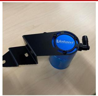
Using a 2.5mm hex key, remove the 3 screws from the top of the catch-can assembly. Align the bracket so that it is approximately at the 8 o'clock position relative to the etch Volant logo atop the catch can and secure using the 3 screws and 2.5mm hex. Do not fully tighten the bolts at this time.
