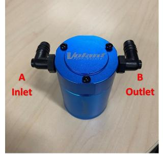
Install both 90 degree barb to 3/8" NPT fittings to the catch can using an 11/16" wrench. The barbed end of the fitting should be facing away from the vertical Volant logo on the catch can body. IMPORTANT: Volant highly recommends using thread sealant of PTFE tape on threaded fittings to prevent any leaks.
