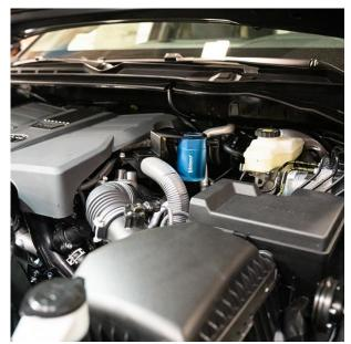
**12.** Reinstall the engine cover by first aligning and inserting the rear pivot points, then lower the front of the cover untill the tabs click into place.
