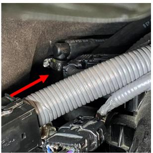
Slide the supplied SAE #6 hose clamp over the rubber PCV line located at the rear of the engine. Insert the 10mm barb portion into the vehicles PCV hose and secure using the SAE #6 clamp and ¼" socket.
