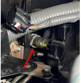
Locate where the PCV hose connects to the intake manifold at the rear of the engine. Loosen the constant tension clamp by squeezing the two tabs together and slide it down the hose. Carefully remove the rubber PCV hose from the fitting and then remove the constant tension clamp.
