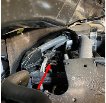
2. Looking at the rear of the engine, from the passenger side, locate the above pictured wiring harness connector. Remove the connector from the bracket, by squeezing the two tabs using a flat head screwdriver from underneath the bracket.
