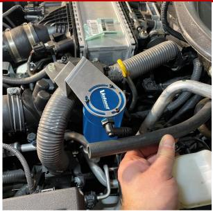
Route the open end of the 24" long x <sup>1</sup>/<sub>2</sub>" hose along the firewall to the B outlet fitting of the catch can assembly. Trim away any excess length from the hose and insert it onto the fitting until the hose is fully seated.
