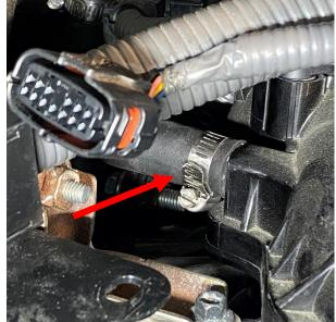
Slide the supplied #6 SAE hose clamp over the smaller 3" long hose. Next, slide the 3" long hose over the PCV fitting on the vehicle intake manifold, ensuring the hose is fully seated on the fitting. Position and secure the SAE #6 hose clamp over the hose and fitting using an ¼" socket.
