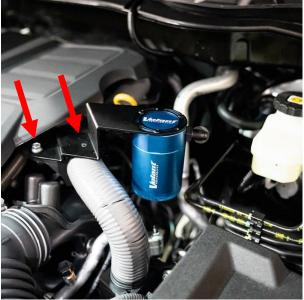
**3.** Align the mounting bracket hole with the threaded hole and plastic tab on the engine wiring harness. Using the bolt removed during step 4 of the removal portion of these instructions, secure the bracket using a 10mm socket and ratchet.
