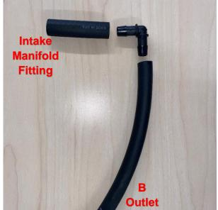
4. Locate the supplied <sup>1</sup>/<sub>2</sub>" 90 degree barbed fitting, one of the two 24" long x <sup>1</sup>/<sub>2</sub>" hoses and the smaller 3" long x <sup>1</sup>/<sub>2</sub>" hose. Connect the two hoses using the fitting, ensuring the hoses are fully seated.
