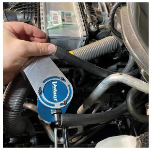
Route the open end of the 24" long x ½" hose along the firewall to the A inlet fitting of the catch can assembly. Trim away any excess length from the hose and insert it into the A inlet fitting until the hose is fully seated.
