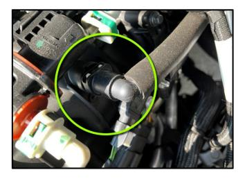
Begin by disconnecting the Factory PCV Line located on the Driver side of the engine by pulling on the grey tabs.
