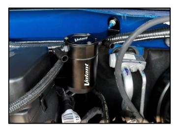
Locate the provided M6 Nut. Secure the Volant Catch Can and Bracket using a 10mm Socket & Ratchet or Wrench and reusing the Factory Stud.
