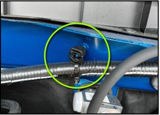
2. On the Driver side of the upper firewall, locate the Plastic Push Nut and Zip Tie. Using a pair of Pliers for cutting, cut the Zip Tie and pull the Push Nut off to expose the Stud on the
