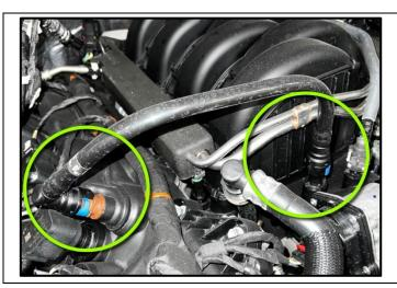
Begin by locating the Factory PCV Line. This line should route from either Valve Cover or Crankcase to the Throttle Body. Typically, these connections are Quick Connect fittings. Squeeze the tabs on the sides of the Quick Connect fittings to release them.
