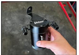
3. Using an 11/16in wrench, install Barbed fittings. **DO NOT OVER TIGHTEN!**
