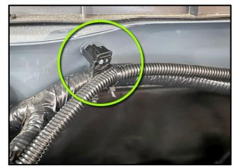
2. On the Passenger side of the upper firewall, locate the Plastic Push Nut and Zip Tie. Using a pair of Pliers for cutting, cut the Zip Tie and pull the Push Nut off to expose the Stud on the
