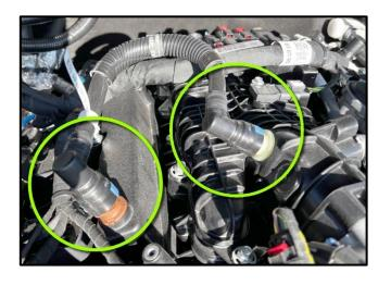
Begin by removing the Factory PCV Line located 1. on the passenger side of the engine by pulling on the blue tabs.
