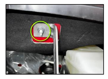
Locate the Nut on the Driver's side firewall that holds the coolant reservoir. Remove the nut using a 10mm Socket & Ratchet or Wrench. This nut will be reused.
