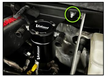
Secure the Volant Catch Can and Bracket using a 10mm Socket & Ratchet or Wrench and reusing the Factory Nut and Stud.
