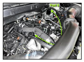
Plug the Quick Connect Fitting on Hose B to to the BLACK fitting on the engine. Next, route Hose B in front of the engine and underneath the intake duct and connect it to Port B of the Volant Catch Can.
