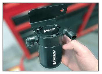
3. Using an 11/16in wrench, install Barbed fittings. **DO NOT OVER TIGHTEN!**
