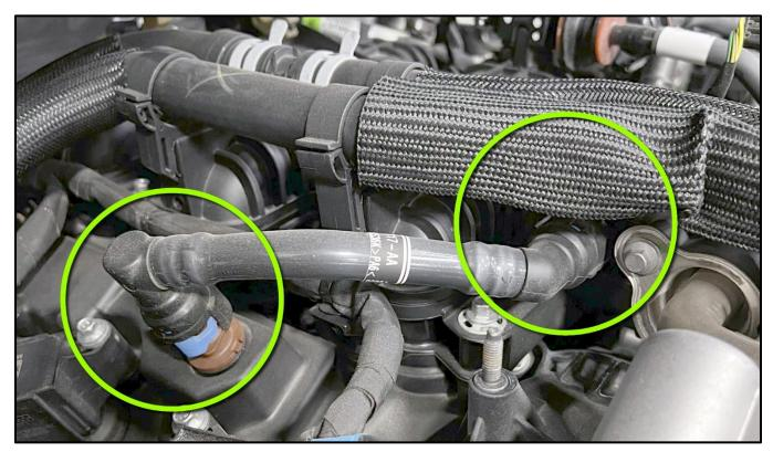
2. On the Passenger side of the engine, locate and remove the Factory PCV line by pulling on the blue tabs
