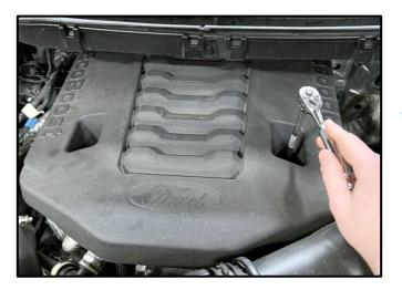
Using a 10mm Socket & Ratchet or Wrench, 1. remove the 2 nuts securing the Factory Engine Cover. Next, pull the Engine Cover forward to remove it from the vehicle.
