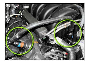
Begin by removing the Factory PCV Line located on the passenger side of the engine by pulling on the blue tabs.
