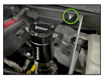
Secure the Volant Catch Can and Bracket using a 10mm Socket & Ratchet or Wrench and reusing the Factory Nut and Stud.
