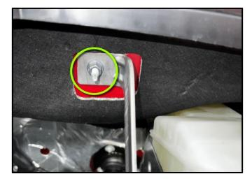
Locate the Nut on the Driver's side firewall that holds the coolant reservoir. Remove the nut using a 10mm Socket & Ratchet or Wrench. This nut will be reused.
