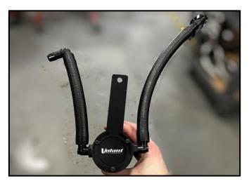
Using an 11/16in wrench, install Barbed fittings. DO NOT OVER TIGHTEN!
