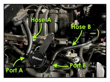
**6.** First connect the barbed fittings to the PCV hose ends. Make sure Hose A connects to the side located on top of the engine and Hose B connects to the side on the front of the engine.
