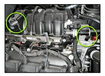
3. On the Passenger side of the engine, remove the Factory PCV Line, in the 2 locations shown.
