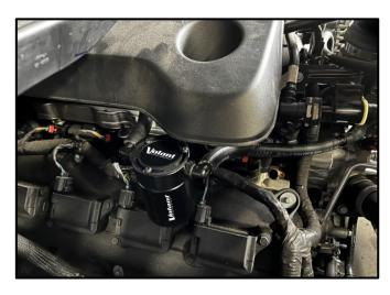
8. Align the hole on the Bracket and Spacer with the Bolt hole that secures the engine cover. When aligned, reinstall the engine cover and thread in the T-30 Torx bolt to the catch can. Reinstall the other T-30 bolt to secure engine cover.
