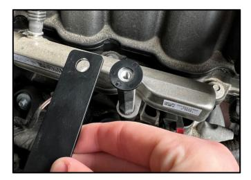
Place the provided spacer between the catch can bracket and the bolt hole.
