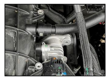
11. Connect Hose B (shorter) to the Intake Manifold (from Step 3) and attach the other end to the 90deg Elbow Fitting in Port B of the Volant Catch Can. See Step 12 for uggested routing.
