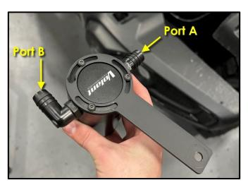
6. Using an 11/16in wrench, install Barbed fittings. DO NOT OVER TIGHTEN!
