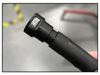
Attach quick disconnect fittings to one end of each of the provided hoses. A mild lubricant or heat may be needed to fully install fitting into hose.
