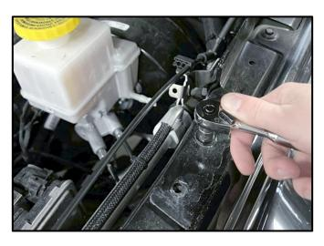
Using a 10mm Socket & Ratchet or Wrench, remove the Factory Bolt located next to the brake fluid reservoir on the Driver's side. Next, install the catch can bracket reusing the Factory bolt to secure the Volant Catch Can and Bracket.
