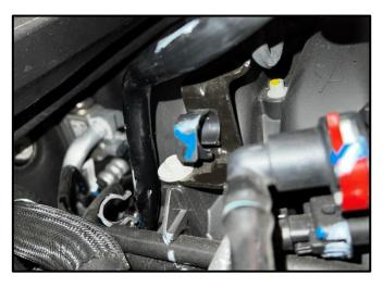
There are 4 clips attached along the Factory PCV line, 2 of them are circled in the image. Detach PCV line from clips and remove the PCV line from the vehicle.
