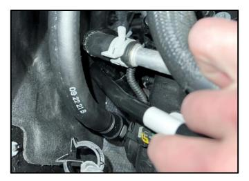
10. Attach Hose A (longer) to the Crankcase on the back corner Passenger side of the engine (from Step 4). Route the Hose along the firewall and underneath the Coolant Reservoir and attach it to the Straight Fitting in Port A of the Volant Catch Can. See Step 12 for uggested routing.
