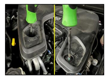
Begin by removing the 2 screws by using a T-30 Torx Driver to remove the Factory Engine Cover.
