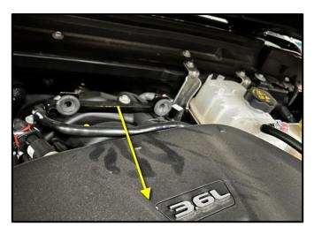
2. Next, pull the Engine Cover forward to remove it from the Grommets.
