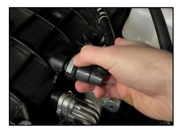
3. Locate the PCV line on Driver's side of the Intake Manifold. Remove the Quick Connect Fitting by squeezing the grey tabs and pulling.
