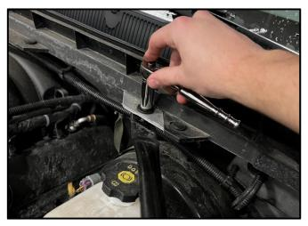
1. Locate the Fender Brace on the Driver's side, above the Brake Fluid Reservoir. Using a 13mm Socket & Ratchet or Wrench, remove the Bolt. Place Catch Can Bracket on top of flat surface and reinstall the Bolt.
