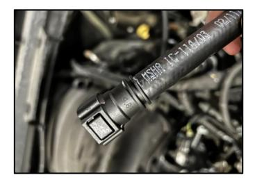
**6.** Attach quick disconnect fittings to one end of each of the provided hoses. A mild lubricant or heat may be needed to fully install fitting into hose.
