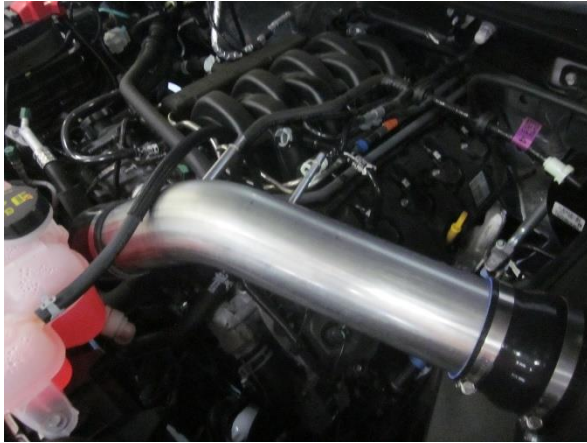
9. Position duct and tighten all clamps with 8mm socket and ratchet.
