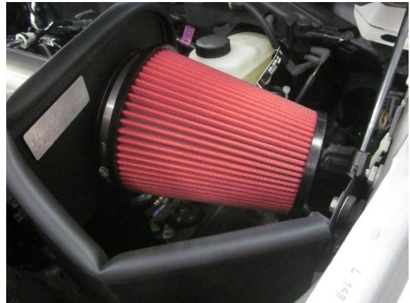
12. Install filter onto filter adapter and tighten clamp with 8mm socket and ratchet.
