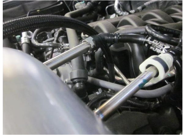
10. Connect the two factory hoses to rear of duct.
