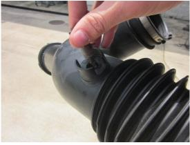
10. Remove the temperature sensor from the factory air duct.
