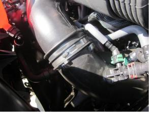
3. Loosen lower factory intake air duct clamp.
