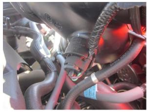
1. Disconnect wiring harness from sensor on rear of factory air duct.
