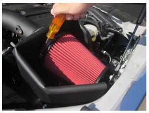
9. Install filter onto adapter and tighten clamp with 8mm socket and ratchet. Place CARB EO label in visible location under hood.
