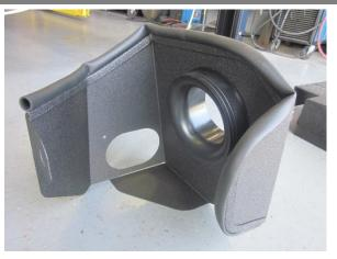
2. Install vinyl trim on Volant metal shield. Add relief cuts at sharp corners to ease installation.
