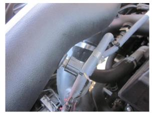
7. Connect wiring harness to temperature sensor.
