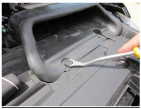
8. Remove the two clips securing the factory air scoop using trim removal tool.
