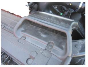
8. Install clips from removal step 8 back into factory location securing factory air scoop.
