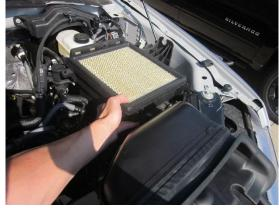
9. Remove the entire lower box and scoop assembly as one piece.
