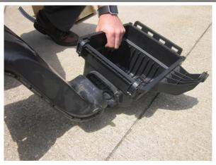
11. Remove bolt securing factory air scoop to lower air box using an 8mm socket and ratchet.
