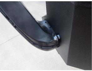
3. Attach factory air scoop to Volant metal shield. Place the ¼" spacer between the scoop and metal shield and use the 6mm x 25 bolt along with ¼" x ¾" flat washer, normal ¼" flat washer, ½" lock washer, and 6mm nut to secure. Tighten hardware with a 10mm socket and ratchet and 10mm wrench.
