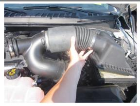
5. Remove factory air duct and lid as one piece.
