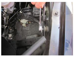
4. Install Volant metal shield into vehicle. Secure shield to vehicle using hardware from removal step 6. The rubber grommet and metal bushing should act as a spacer for the shield. Tighten with a 13mm wrench.
