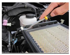
7. Remove the two plastic wire retention clips from the rear of the factory air box using a trim removal tool.
