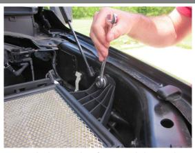
6. Remove bolt securing factory air box using 13mm wrench.
