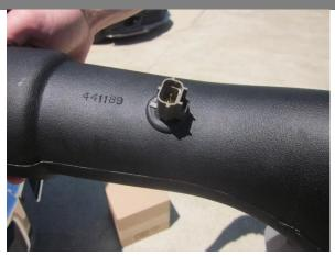
5. Insert factory temperature sensor from removal step 10 into Volant air duct grommet.
