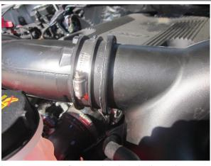
2. Loosen upper factory intake air duct clamp.
