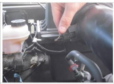
1. Disconnect harness from the air temperature sensor.
