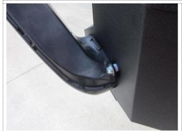
Install stock air scoop to bottom of VOLANT APEX heat shield using the 6mm x 25 bolt, 1/4" spacer, lock washer, flat washer, and 6mm nut.
