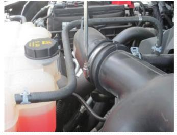
2. Loosen the rear clamp on the upper air intake tube.
