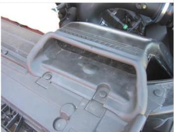
8. Reinstall factory fender plastic pins into the air inlet opening from Removal Step 8.
