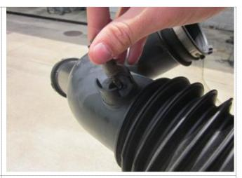
**10.**Remove the air temperature sensor (ATS) from the factory air duct removed in Removal Step 5. Save the sensor for the re-installation in the VOLANT APEX air duct.
