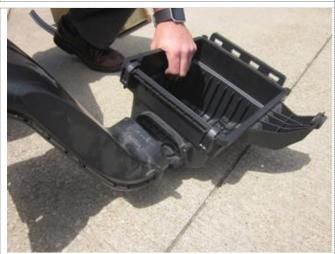
12.Once the fasteners have been removed from the air scoop, separate the scoop and the air box.
