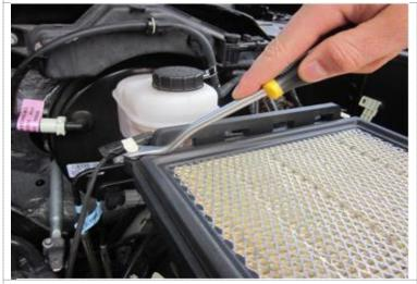
7. Using a nail puller, or a flat blade screwdriver, gently remove the two plastic wire retention clips from the back of air box.
