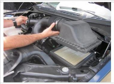
5. Disconnect the air tubes, lift the lid and remove the air duct and air box lid assembly as one piece.
