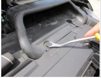
8. Using a fender clip removal tool or a flat blade screwdriver, remove the two plastic clips from the factory air scoop. Save the plastic clips for the installation of the VOLANT APEX heat shield.
