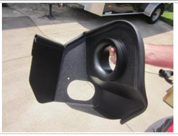
2. Install the trim strip on VOLANT APEX heat shield. Add a relief cuts with the metal cutting snips where necessary to allow trim to form around sharp bends. Use slip joint pliers to crimp the trim strip onto the heat shield.
