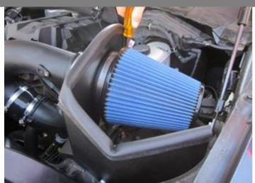
9. Install the VOLANT Pro-5 filter (or DryTech 3D filter) onto the filter adapter and tighten the clamp with a using a flat blade screwdriver or a 5/16" nut driver.
