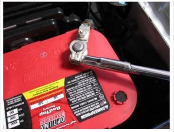
11.Reattach the negative battery cable and recheck all connections before driving. Retighten all clamps after 500 miles.
