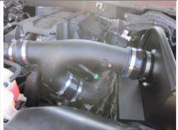
6. Slide two #064 clamps onto the 4" straight sleeve hose and place onto the lower factory intake tube. Place two #064 clamps on the 4" hump hose and slide onto the filter adapter. Slide one #048 clamp and one #056 clamp onto the silicone reducer hose and place onto the factory air duct. Once all of the hoses are in place, install the VOLANT APEX air duct onto the hoses, and using a flat blade screwdriver or a 5/16" nut driver, tighten all of the clamps.
