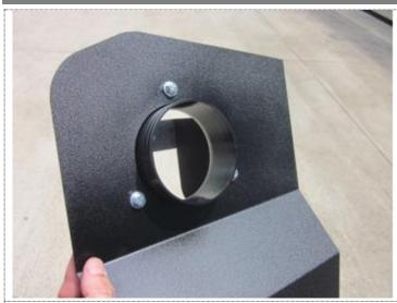
1. Begin assembly by bolting the filter adapter to heat shield using supplied 6mm x 14 bolts, 1/4" lock washers, and 1/4" flat washers.
