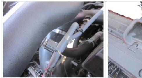
7. Reattach the ATS wiring harness to the sensor.
