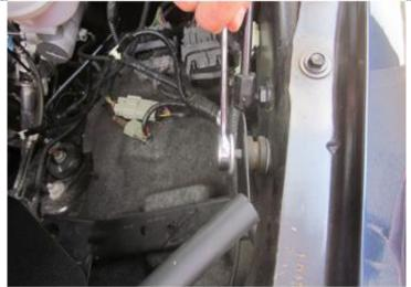
4. Insert heat shield into the space used by the original air box. Bolt the side of heat shield to vehicle using the factory 13mm bolt and rubber washer from Removal Step 6.
