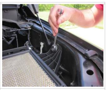
6. Using a 13mm open/closed box end wrench, remove the bolt holding the air box to the vehicle. Remove the rubber grommet and metal washer and save for installation of the VOLANT APEX heat shield.
