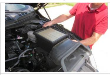
9. Lift the lower air plenum and the air scoop straight up. Remove the assembly from the vehicle.
