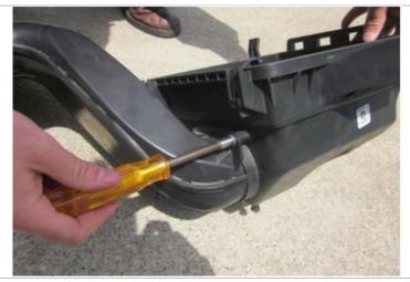
11.Using an 8mm nut driver or socket, remove the factory air scoop from the bottom of the air box.
