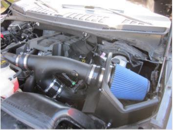
**INSTALLED VOLANT APEX 319635 KIT**
