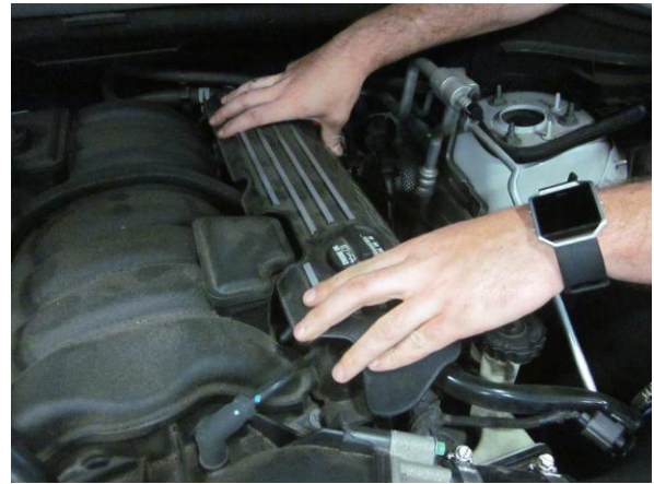
26. Re-install engine cover.
