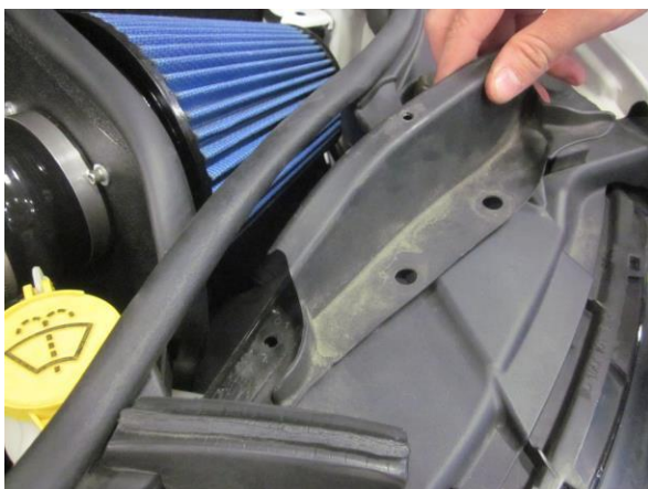
29. Remove factory air dam.
