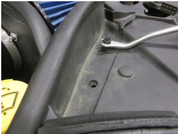
27. OPTIONAL: You may remove the factory air dam to increase air flow to your intake system. Remove the two plastic clips.
