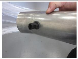
Install supplied rubber grommet into Volant air duct. Install factory ATS from removal step 8 into grommet.
