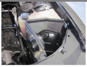
6. Place Volant shield assembly into vehicle.
