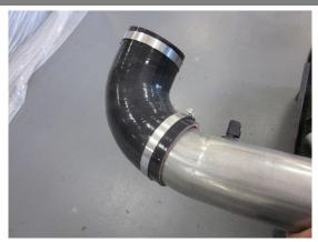
11.Place straight sleeve onto end of Volant duct along with two #60 clamps placed loosely.
