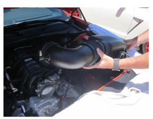
7. Pull factory air duct off throttle body and lift entire factory intake up and out of vehicle.
