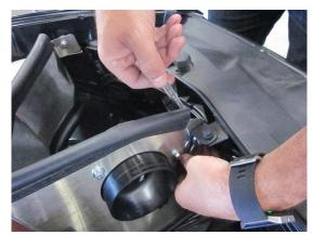
Tighten shield hardware from step 4 using two 10mm wrenches.
