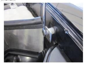
7. Place spacer between shield and inner fender and insert 6mm x 30 bolt with ½" lock washer and ½" flat washer. Tighten bolt with 10mm socket and ratchet.
