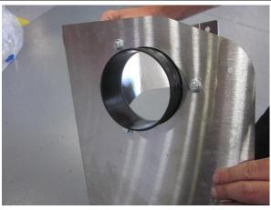
2. Bolt filter adapter to Volant shield with three 6mm x 16 bolts, 1/4" lock washers, and 1/4" flat washers using 10mm socket and ratchet.
