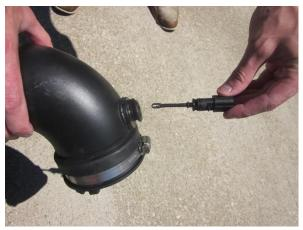
8. Remove ATS from factory air duct.
