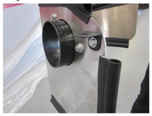
4. Loosely assembly bracket to shield using 6mm x 16 bolt, ½" lock washer, two ½" flat washers, and 6mm nut.
