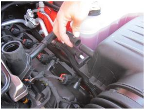
5. Disconnect vacuum hose from factory air box and engine.
