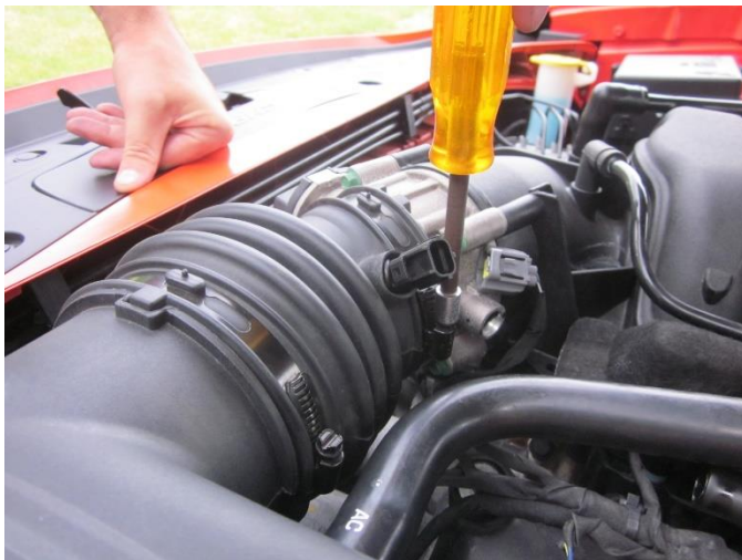
3. Loosen clamp securing factory air duct to throttle body using an 8mm socket and ratchet.
