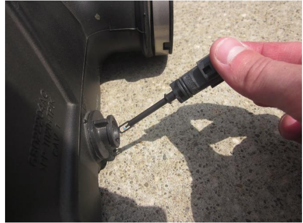
12. Remove ATS from factory air duct.
