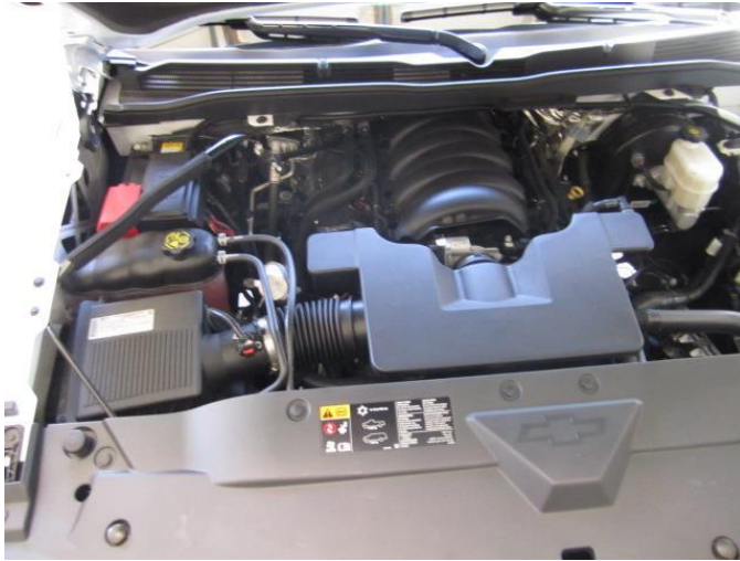
1. Stock air intake system before uninstallation.
