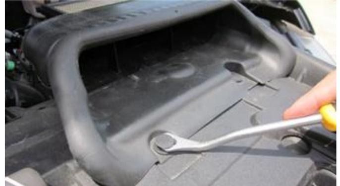
**6.** Remove the two plastic clips from the factory air scoop. Save clips for **Install Step 5**.
