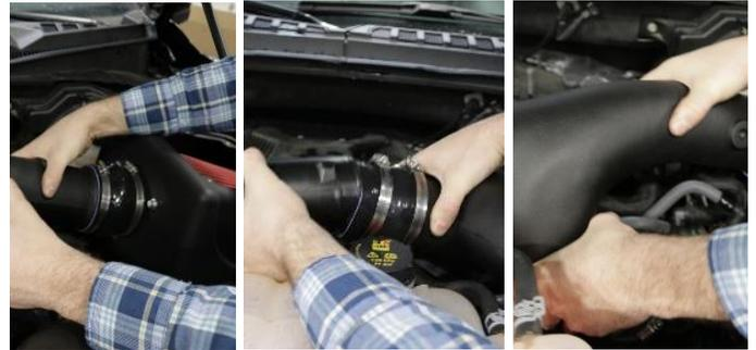
13. Install Volant air duct into vehicle by placing the hump hose onto the filter adapter. Then place reducer onto the upper stock inlet. Rotate duct down and into the straight sleeve.
