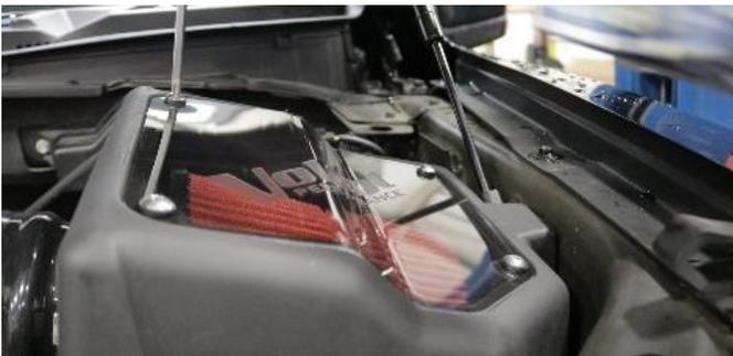
16. Install lid using provided 4 truss head screws with rubber washers and Philips head screwdriver.
