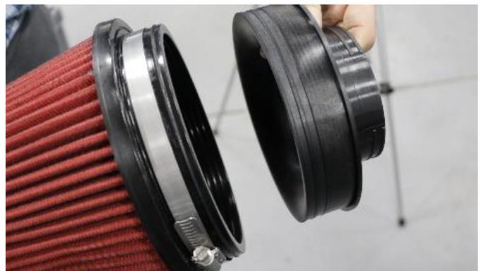
6. Place the filter clamp on the filter and insert the filter adapter as shown. Do not tighten clamp yet.
