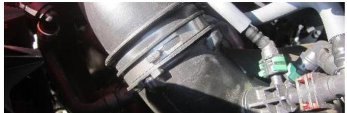
1. Disconnect the harness from the air temperature sensor on back side of factory air duct.
