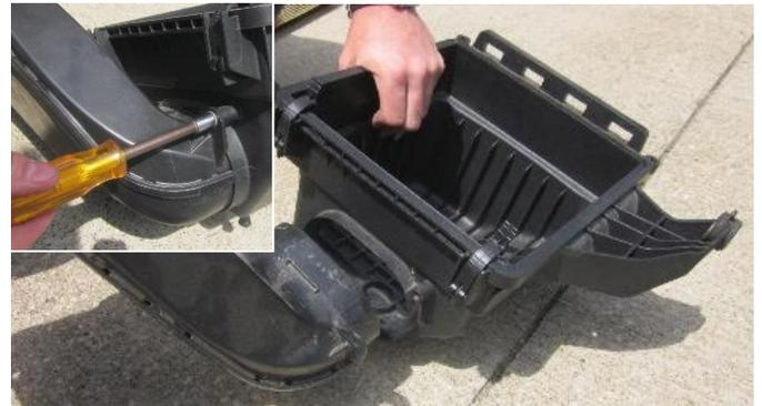
**8.** Remove the bolt attaching the scoop to factory air box using an 8mm socket. Remove the factory air scoop from the bottom of the air box.
