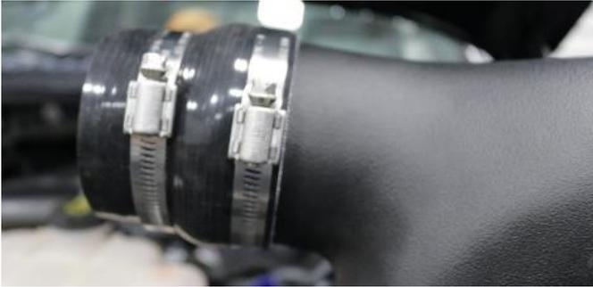
12. Insert larger end of reducer onto Volant air duct using #56 clamp. Place #48 clamp on the smaller side. Tighten #56 clamp only using a ratchet and 8mm socket or flat head screwdriver.
