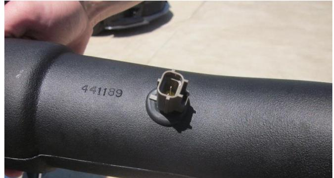
9. Install air temp sensor from **Removal Step 9** with the tab facing the closer end of the duct.
