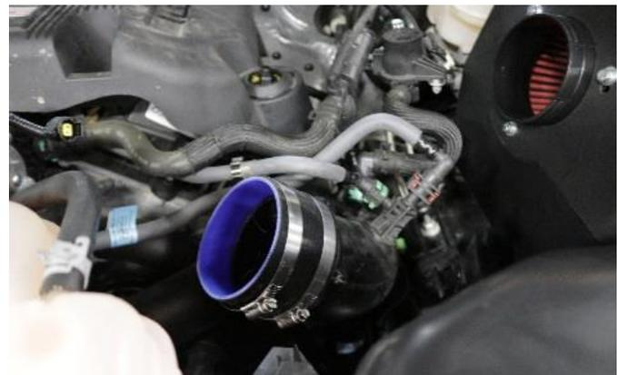
11. Install the straight sleeve onto lower factory inlet with #64 clamp. Tighten clamp using a ratchet and 8mm socket or flat head screwdriver. Leave clamp on open end of straight sleeve loose.
