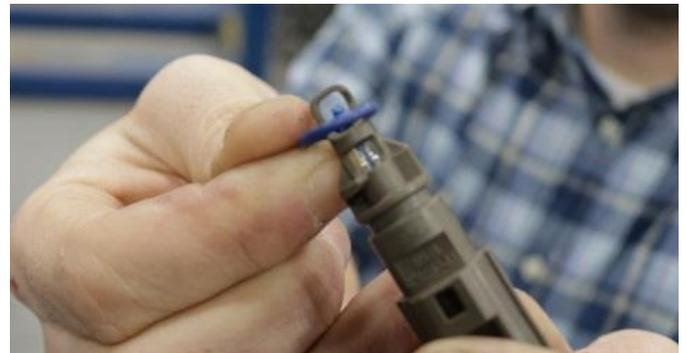
**10.** Remove O-ring from the temp sensor.
