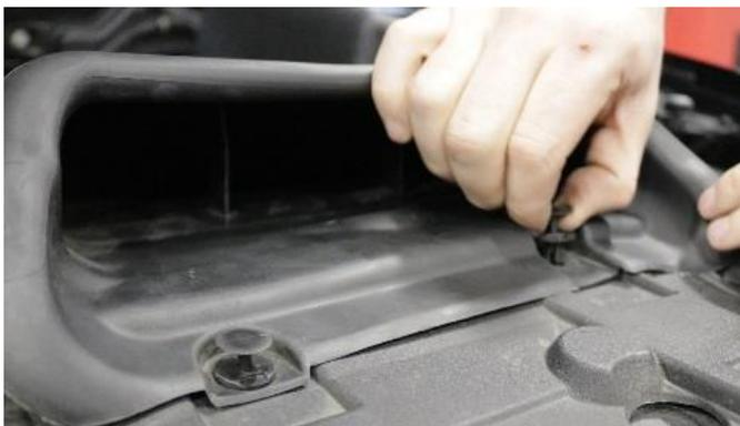
5. Reinstall factory scoop and attach with clips from **Removal Step 6**.
