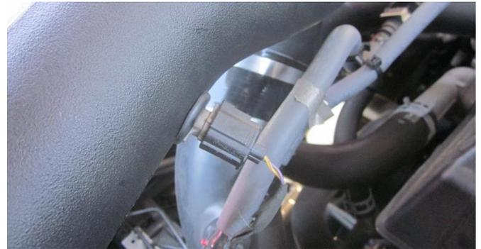
15. Clip wiring harness on air temperature sensor.
