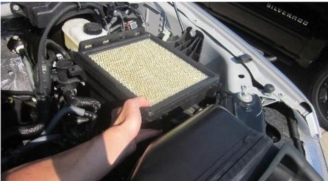
**7.** Remove the bottom box assembly by pulling it up and out. Remove the rubber grommet and metal bushing from factory air box. Save for **Install Step 1**.
