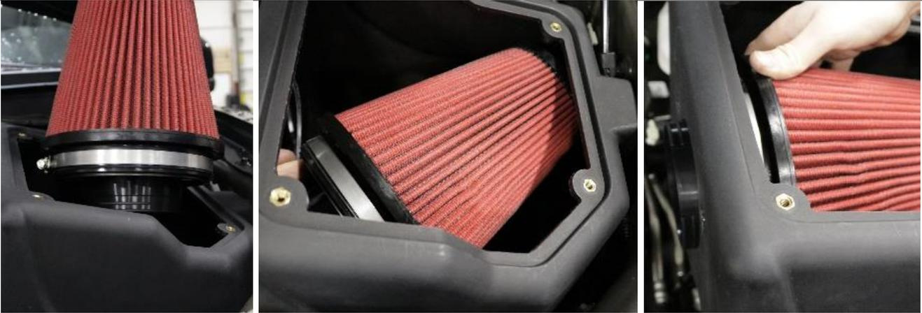
7. Insert the filter into the air box with the adapter side down. Rotate the top of the filter down into the air box and rotate the filter around and push the adapter through air box.
