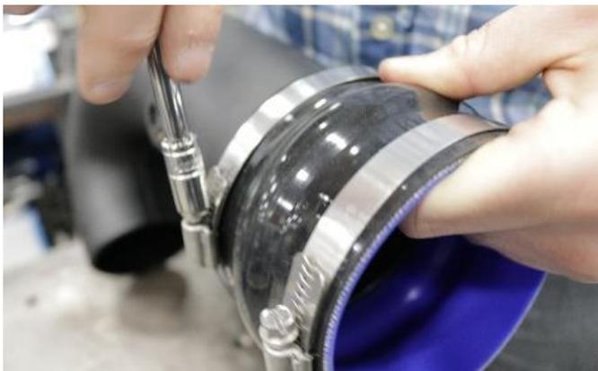
10. Install the hump hose onto the Volant air duct along with two #64 clamps and tighten using a ratchet and 8mm socket or flat head screwdriver. Leave clamp on open end of hump hose loose.
