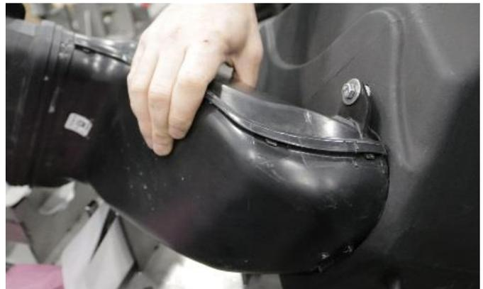
2. Install factory scoop to Volant air box using provided 6mm-25 bolt with flat washers, lock washer, spacer, and nut using 10mm socket or wrench..
