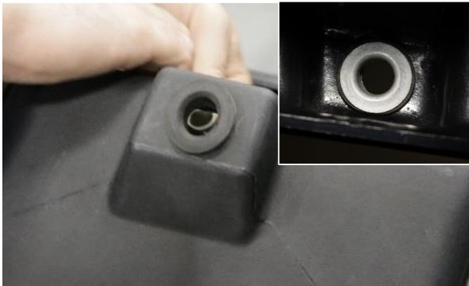
1. Insert the factory grommet from **Removal Step 7**, then install the metal bushing into grommet from inside box as shown.
