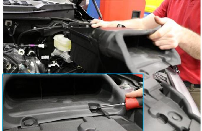
8. Remove the two clips holding the factory scoop using a pry tool. Save clips for **Install Step 5**. Remove scoop and air box assembly from vehicle.
