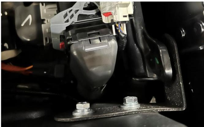
7. Insert push clip on factory wiring harness mount into hole on bracket
