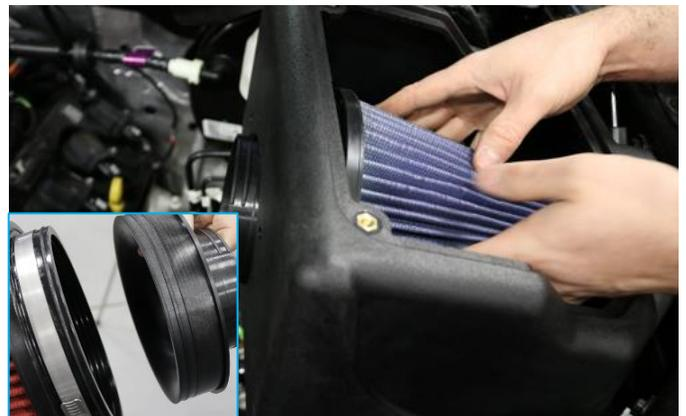
8. Install filter adapter onto Volant air filter, then place air filter into Volant air box.
