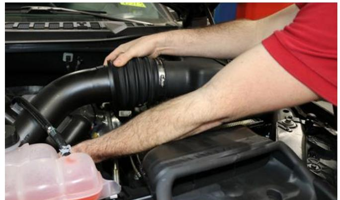
4. Unclip the air box lid and remove the factory duct and lid assembly as one piece.
