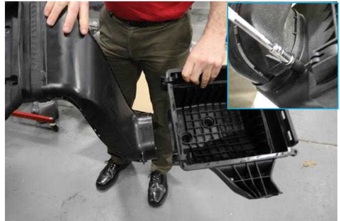
10. Remove the bolt holding the factory air scoop to the air box using an 8mm socket. Separate the scoop from box and save it for **Install Step 3**.
