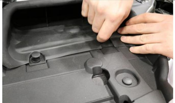
6. Re-install the factory scoop with clips saved from **Removal Step 8**.
