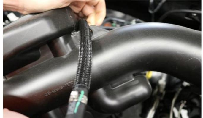
2. Release the coolant hose from the factory air duct.
