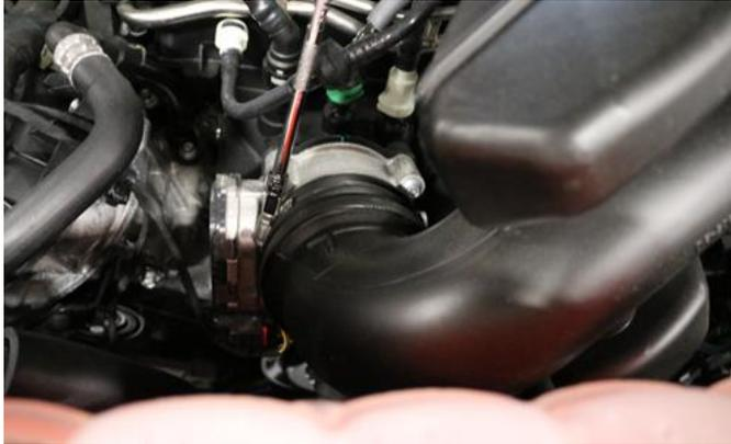
1. Loosen the throttle body clamp using a 7mm socket.
