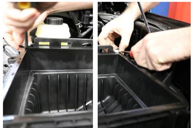
6. Use a pry tool to remove the three wire retention clips.
