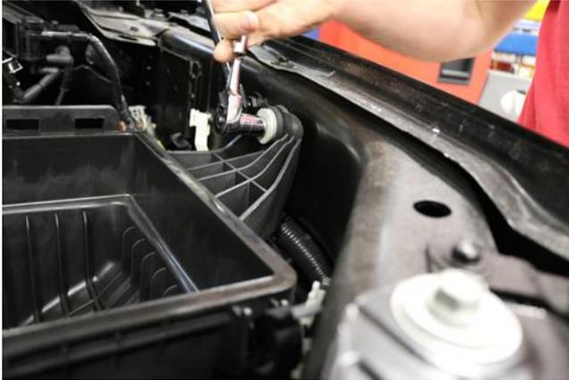
7. Use a ratchet and 13mm socket or wrench to remove the bolt holding the air box to the vehicle. Save bolt for **Install Step 4**.
