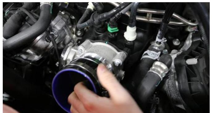
10. Install two #56 clamps onto the straight sleeve and place the straight sleeve on the throttle body.
