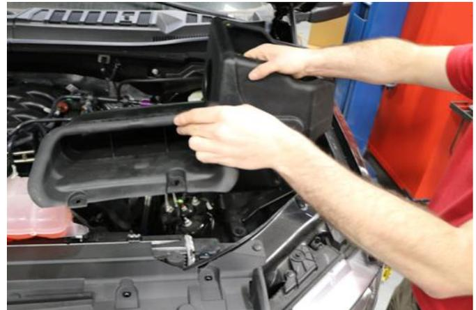
4. Install the factory air scoop, and Volant air box into vehicle making sure to place the studs on the bottom of the air box into factory grommets.
