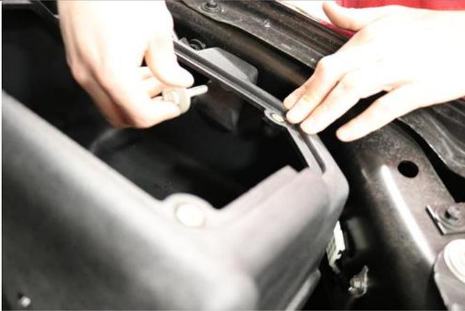
5. Use the bolt saved from **Removal Step 7** to attach the Volant air box to the fender with a 13mm socket.
