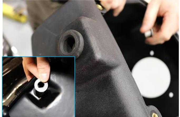
2. Put the metal bushing and rubber grommet from **Removal Step 9** into the Volant air box.
