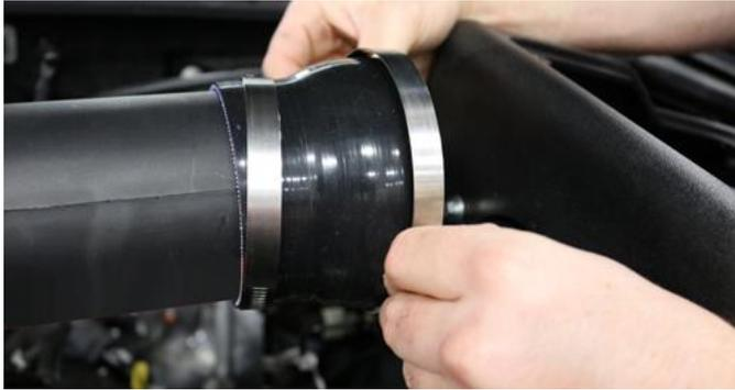
11. Install one #56 clamp on small end of the reducer, and one #64 clamp on larger end of reducer. Place small end of reducer onto straight end of Volant air duct.
