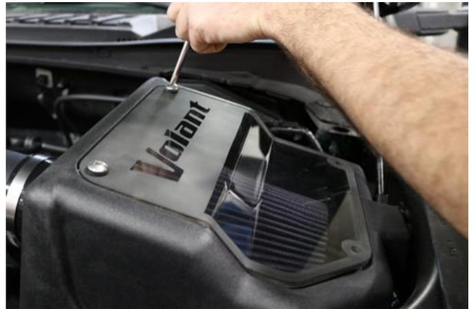
14. Install the Volant lid using the provided 4 truss head screws with rubber washers and Philips head screwdriver.
