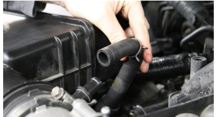
2. Disconnect factory vent hose from stock air duct.
