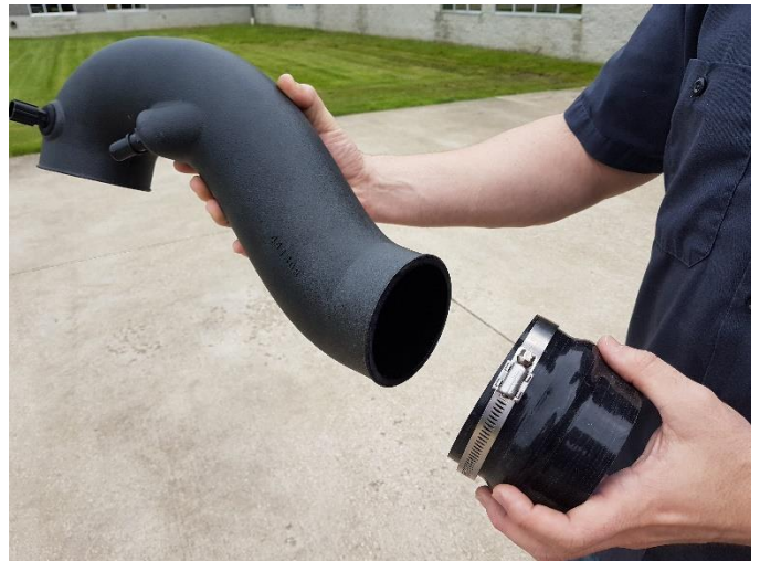
13. Insert a 4" Clamp onto one end of the hump hose and slide it onto the duct.
