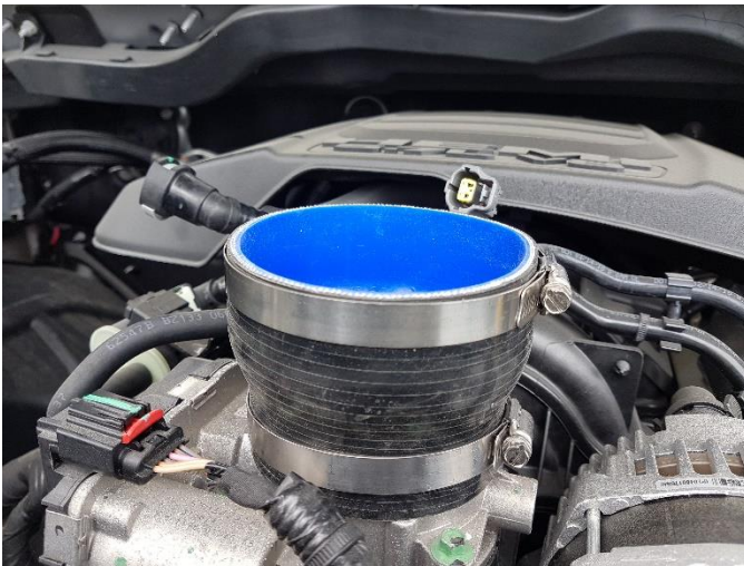
12. Insert another 4" clamp onto the other end of the reducer as shown.
