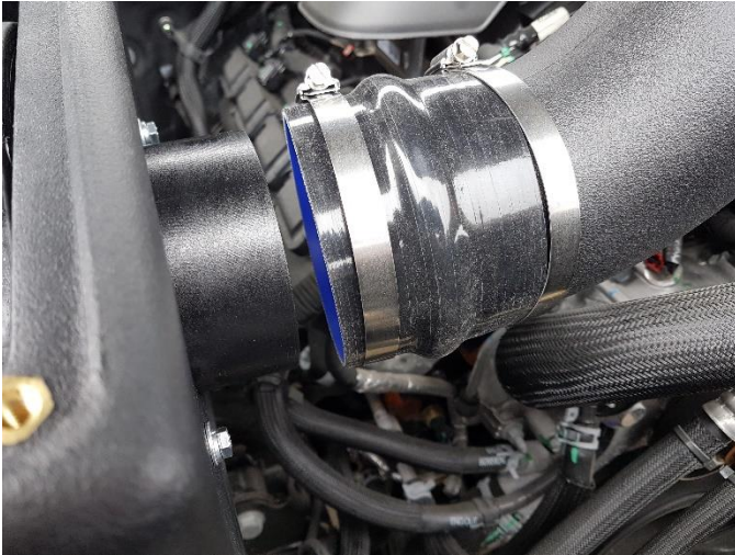
14. Insert the last 4" Clamp onto the other end of the hump hose and slide the duct onto the box assembly.
