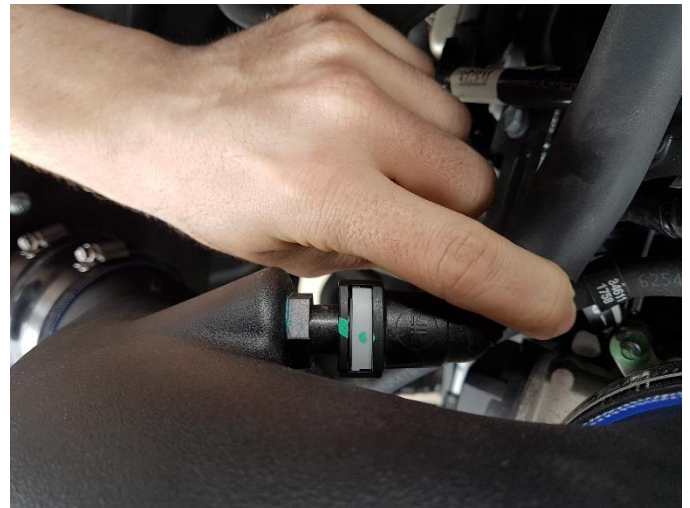
17. Connect the crank case vent hose to the fitting until it clicks.
