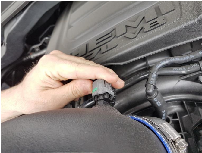
16. Plug in the air temperature sensor making sure that the sensor doesn't get rotated.
