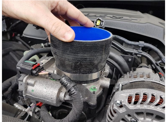
11. Insert the reducer with the clamp onto the throttle body and tighten the clamp using a 8mm socket and ratchet.
