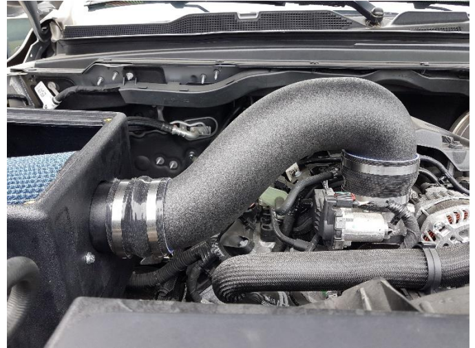
15. Slide the other end of the duct into the reducer on the throttle body,.
