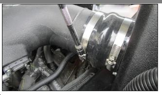
**8.** Adjust duct fitment as necessary and tighten all four clamps using a ratchet and 8mm socket.
