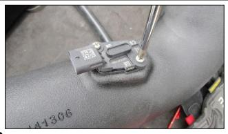
**2.** Install sensor into Volant air duct. Secure using the two supplied screws and a Philips head screwdriver.
