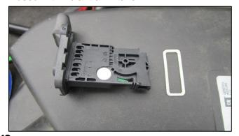
**12.** Remove factory gasket from MAF sensor.
