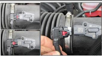
Pull red tab on MAF sensor wiring harness. Squeeze black clip behind red tab to release wiring harness and pull harness from the sensor.
