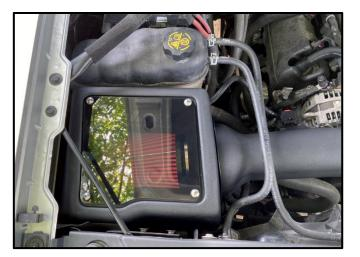
**14.** Using a Phillips Head Screwdriver, install the Volant Intake Lid. Start by loosely installing the upper left screw (round hole) first. The other 3 screws are in a curved slot to help with alignment.
