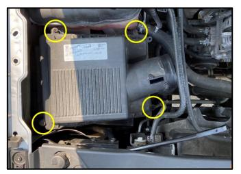
Using an 8mm Socket & Ratchet or Wrench, remove the 4 bolts holding the Factory Air Box Lid from the Base. These will not be reused.
