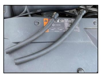
Locate the 2 Hoses and 2 Quick Connect Fittings. Press the fittings into one end of the hoses, as shown.
