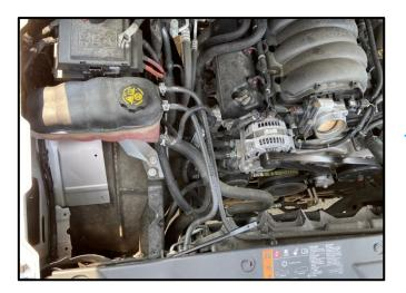
12. Remove the Factory Air Box Tray from the Vehicle.
