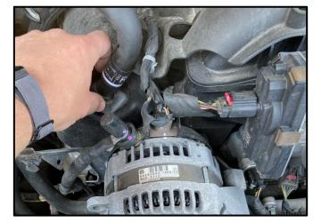
After the Factory Air Duct is removed, go back to the Factory Hoses. Squeeze the Grey Tabs, pull up and remove the hoses. These will not be reused.
