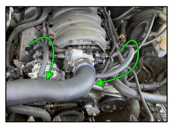
Insert the Quick Connector of the Long Hose onto the Valve Cover Port on the Driver's side and the Quick Connector of the Short Hose onto the Valve Cover Port on the Passenger's side. Once those are connected, route the hoses to the fittings in the Air Intake Duct, as shown.
