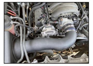
6. Next, install the assembled Air Intake Duct into the vehicle. Begin by sliding the large end into the opening in the Air Intake Box. Next, rotate and move the Air Intake Duct until the Hose or Reducer are aligned with the Throttle Body. Then slide the Hose or Reducer on to the Throttle Body and arrange the Hose Clamps as shown. On the 6.2L, the larger clamp goes on to the Throttle Body. Once everything is properly aligned, use an 8mm Socket & Ratchet or Wrench to secure the Hose Clamps.
