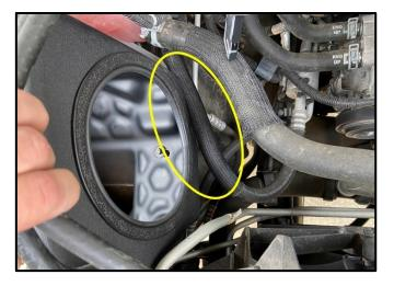
Before tightening the mounting bolts, ensure the hose shown in the oval is not under the Air Intake Box. This will hold the Volant Air Intake Box up and not in place.
