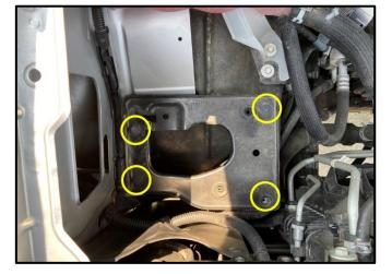
Using a 10mm Socket & Ratchet or Wrench, remove the 4 bolts holding the Factory Air Box Tray from the Vehicle. Store them in a safe location. 3 of the 4 screws will be reused in Installation Step 3.
