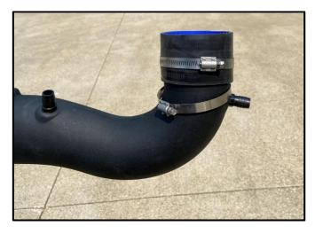
Locate the Volant Air Intake Duct, the 2 Hose Clamps, the 2 Thread to Barb Fittings and either the Ø4in to Ø3.5in Reducer (6.2L) or Ø3.5in Hose (5.3L) (shown). Assemble the parts to the Air Intake Duct as shown. The Thread to Barb Fittings should be tightened until they are tight and flush to the mating surface on the Air Intake Duct. The hose clamps should be loose at this time.
