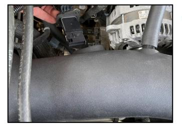
9. Locate the MAF Sensor Gasket and install it onto the MAF Senor removed in from Removal Step 3. Next, slide the MAF Sensor and Gasket into the opening in the back of the Air Intake Duct. The Flat Side goes up and the screws will only align one way. Then locate MAF Screws from the Hardware Kit and use a Phillips Screwdriver to secure the MAF Sensor to the Air Intake Duct. Once the MAF Sensor is secured, reconnect the Wire Harness and push the Red Locking tab down.
