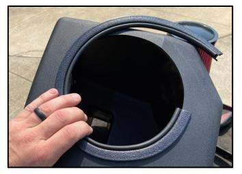
1. Locate the Volant Air Intake Box and the Box Opening Seal. Starting on the bottom of the opening, press the Seal around the opening.
