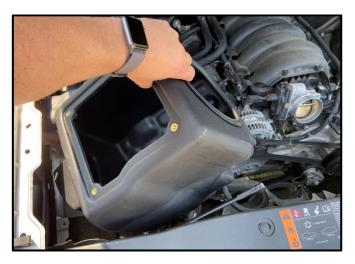
2. After the Seal is installed, install the Air Intake Box into the vehicle. This is done by sliding the Side Inlet Duct through the opening in the Fender and the Lower Inlet Scoop through the opening above the fender.
