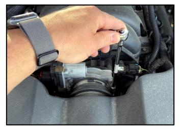
Using an 8mm Socket & Ratchet or Wrench, loosen the Hose Clamp connecting the Factory Air Duct to the Throttle Body. This will not be reused.
