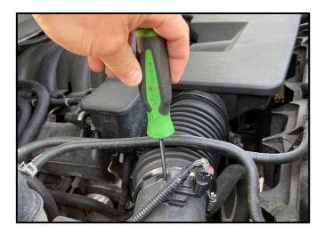
Using a T15 Torx Driver, remove the Factory MAF Screws. These will not be reused. Next, disconnect the Mass Air Flow (MAF) Sensor from the Wire Harness by pulling the red clip up and then squeeze the sides of the Wire Conncetor to release it. Carefully remove the MAF Sensor and store it in a safe location. It will be reused in Installation Step 9.
