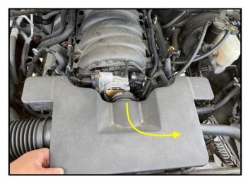
Pull the Factory Duct toward the front of the vehicle to disconnect it from the Throttle Body. Next, pull the Factory Duct toward the Driver's side to disconnect it from the Factory Air Box. Then lift the Factory Air Duct out of the vehicle.
