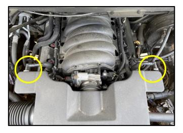
Locate the Factory Quick Connections on the rear of the Factory Air Duct. Squeeze the Grey Tabs and pull the Connections off the Factory Duct and rotate the Stock Hoses out of the way.
