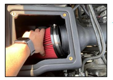
Next, locate the Filter (DryTech 3D shown). Insert the Filter into the Air Intake Box with the open side up. Turn the smaller end toward the fender, and then slide the open end onto the Air Intake Duct. Rotate the Filter or Clamp so the bolt on the Filter Clamp is accessible and use an 8mm Socket & Ratchet or Wrench to secure the Filter Clamp.
