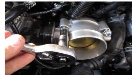
6. Install the spacer with the gasket between the throttle body and the spacer.
