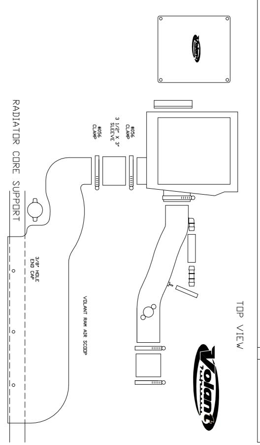
NOTE: REMOVE ALL SIX FACTORY PUSH PINS FROM THE RADIATOR CORE SUPPORT AND REMOVE PLASTIC COVER. PLACE THE VOLANT RAM AIR SCOOP OVER THE CORE SUPPORT AND FASTEN WITH 3 FACTORY PUSH PINS.
