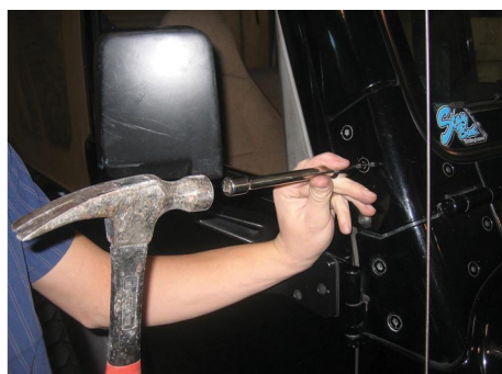
5. Remove the two top counter sink bolts from the front windshield bracket with a torx key #40 Note: In order to loosen the bolts, tap them lightly with a hammer to loosen the Loc-tite.
