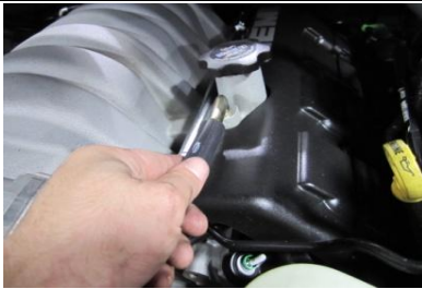
20. Attach the breather hose to the crankcase vent hose and the motor.
