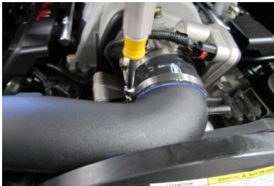
19. Tighten the clamps holding the duct to the filter and the throttle body.
