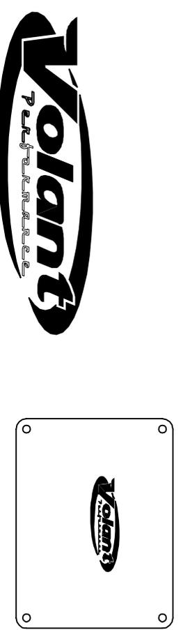
**FRONT VIEW** (4) 1/4"-20 TRUSS HEAD SCREWS (4) 1/4" RUBBER WASHERS
