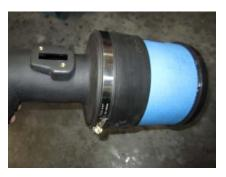
9. Clamp the Filter onto the Volant air duct.
