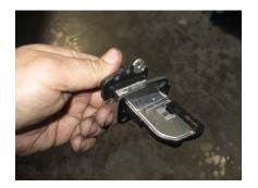
12. Replace the factory sensor gasket with the supplied Volant gasket.
