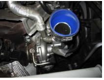
14. Attach the 3 to 2.5 reducer onto the inlet
