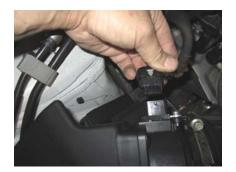
3. Disconnect the MAF sensor harness from the MAF sensor.
