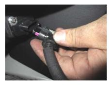
17. Attach the MAF sensor harness and negative battery cable.
