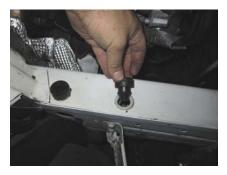
8. Press the rubber mounts back into the stock location.
