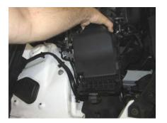
5. Remove the factory air box by pulling up and out.
