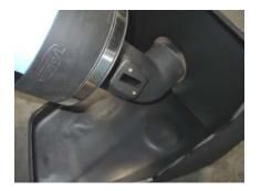
10. Press the duct through the hole in the air box.
