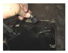
7. Remove the factory rubber mounts from the stock air box.
