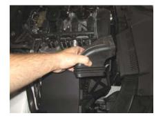
4. Remove the air intake ducting from the factory air box.
