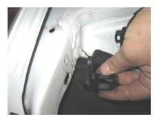
6. Remove the factory bracket assembly from the fender.
