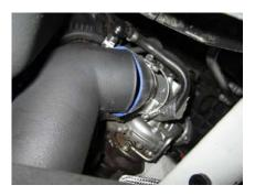
16. Attach the air duct to the reducer using the #48 clamp
