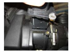
11. Using the T-20 Torx bit remove the factory MAF sensor.
