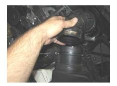
2. Loosen the clamp holding the factory air duct to the factory box.
