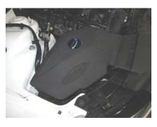
15. Press the Volant box into the factory rubber grommets and into the factory scoop.
