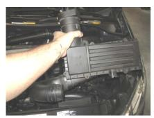
Remove the factory air box by pulling up and releasing it from the factory rubber grommets.
