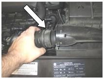
Remove the duct from the air inlet base.
