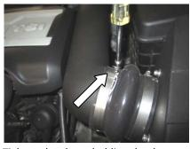
Tighten the clamp holding the duct to the hump hose.
