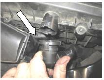
Disconnect the vent pipe from the factory air box.
