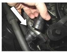
Press the 1" fitting into the factory vent hose, you should hear it click into place.
