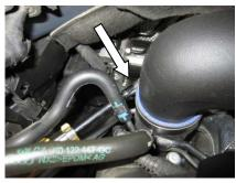
Press the Volant air duct into the hump hose and sleeve. Tighten the clamp holding the sleeve to the duct.
