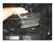
Remove the 2 torx bits holding the air inlet box to the core support than remove the box.
