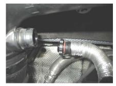
Disconnect the vent pipe from the air duct.
