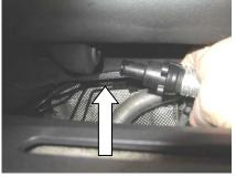
Press the hose adapter into the vent hose until it clicks and press into the rubber grommet.
