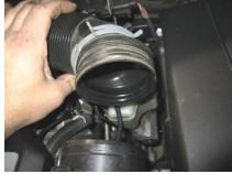
Remove the factory air duct from the factory MAF adapter.
