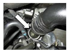
Loosen the clamp holding the air duct in place and lift up on the air duct.
