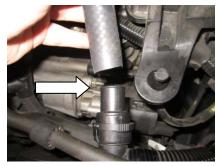
Press the 1" hose onto the adapter.
