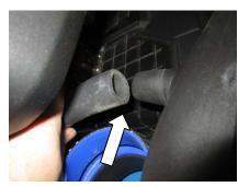
Press the open end of the 1" breather hose onto the Volant duct.
