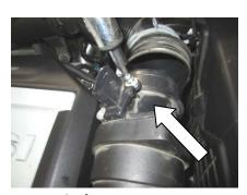
Remove the factory MAF sensor.
