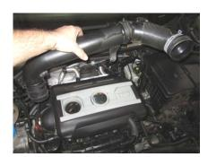
Remove the factory air duct.
