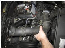
8. To remove the resonator box you will need to remove the two 13mm bolts from the frame. After the box is removed reinstall the skid plate
