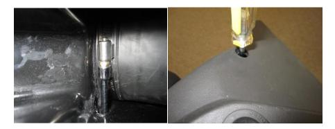
10. Press the factory rubber grommets into the predrilled holes on the bottom of the air box. Press the Volant box onto the factory mounting studs.
