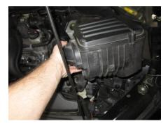
4. Using a torx bit remove the two screws holding the factory air inlet scoop.
