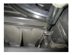
5. Remove the lower ducting and remove the scoop.
