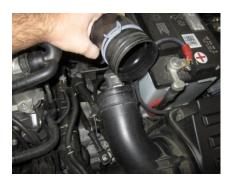
3. Pull up on the factory air box and remove it from the engine compartment.
