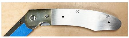
Align right liner over pivot, stop pin and stand offs of assembly and secure with remaining stop pin screws.
