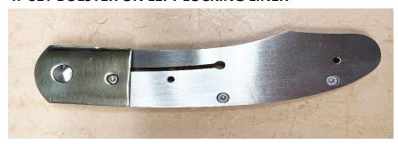
Attach one side of the bolster to the left locking liner by inserting the female pivot pin and screwing the bolster with the medium screw.
