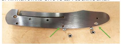
Each locking liner has two stand off holes. Attach the stand offs using the two drilled and threaded stand offs and four smallest screws. The screws go into the countersunk side as shown above.
