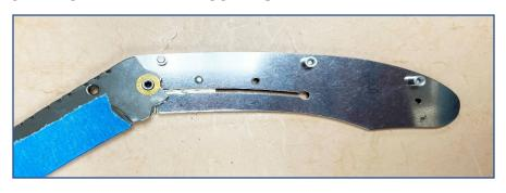
Place the blade over the pivot pin and bushing. Adjust the lock as needed to fit blade securely. Place remaining bushing onto pivot.
