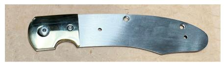
Attach bolster to right liner using remaining bolster screw and insert male pivot pin.
