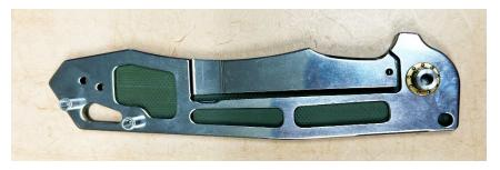
Start with the right handle (the one with pocket clip screw holes) and the liner with the locking mechanism.
