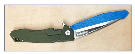
Place remaining handle on top and set liner holes onto stop pin and stand offs. Liner and handle will lay flat against each other when set correctly.
