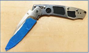
Carefully place the blade onto the pivot pin. Adjust the axis lock to make space for the blade to set fully down on the pivot pin. Put remaining bushing over pivot pin.
