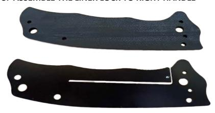
Start with the right handle (the one with pocket clip screw holes) and the liner with the locking mechanism.
